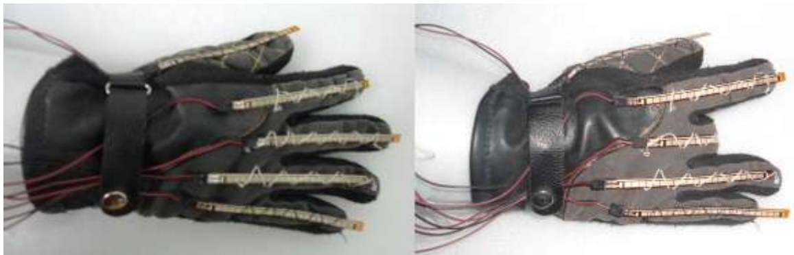
Fig. 2.4. Flex Sensors mounted glove and default unflexed state and flexed middle finger.
